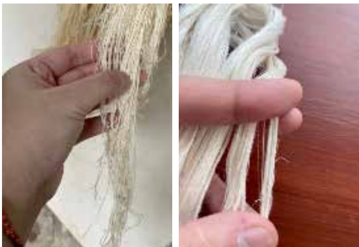
Figure 8: The Rest of The 'Cotton' Processing of Pineapple Fibers on the Decorticator Machine Source: Author,2021
